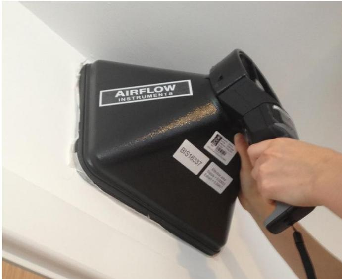
Figure 8. Testing of airflow rates (Source: Gráinne McGill)
