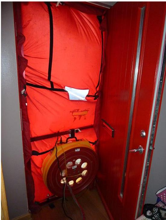
Figure 2. Airtightness testing (Source: MEARU)
